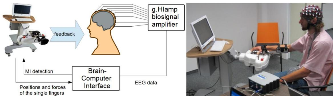
Figure 1: Left: schematic workflow. The device reads the brain signals and sends the classification result to the rehabilitation robot. Right: Photograph of the setup.
