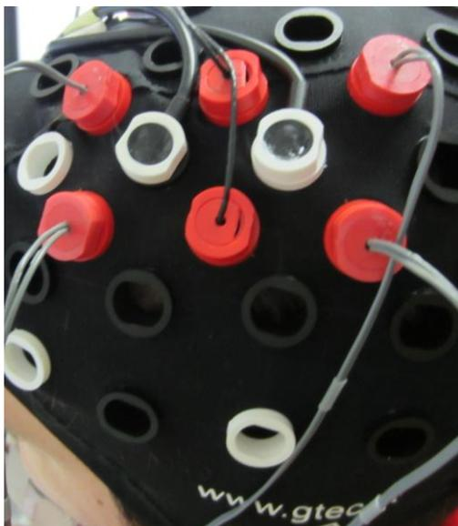
This picture shows the placement of the optodes and electrodes over the left motor cortex. The red optodes in the middle are the sources of the NIRScout device and the white ones are the detectors. The red electrodes in front and back are EEG channels 5 – 8.
