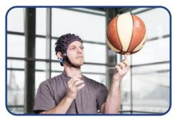
g.Nautilus records up to 64 EEG channels at the highest possible signal quality and with the lowest movement artifacts, due to active electrode technology. This makes the device usable even for difficult experimental settings such as sports activities.
